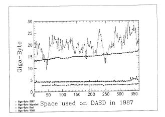
The figure shows the used space during 1987. Space allocation is kept constant during long periods on USERxx and VSAMxx disks (see the lower two polygons: 'Giga-Byte Real' and 'Giga-Byte VSAM') The amount of migrated data space is constantly growing about 32 per cent during 1987 (see the upper polygon: 'Giga-Byte Migrated'). Allocation of temporary data sets varies according to the experimenters' needs (see the middle polygon: 'Giga-Byte SERV').
